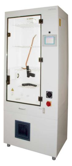
The Cyanoacrylate Fuming Chamber with the new **Touch Panel** can be used to secure traces on all objects with non-porous surfaces.
